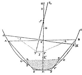
Figure 3: BOUGUER's diagram of the metacenter, [2], fig. 54.
