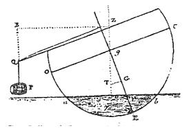
Figure 4: BOUGUER's diagram of an inclining experiment, [2] fig. 55.
